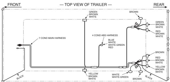
A warning decal, as shown on the previous page, is located on the front of each trailer. You may trace individual electrical circuits by the wire colors indicated. Refer to the schematic drawing and the decal for conductor numbers and wire colors.
